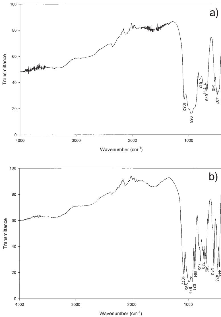
FIG. 2. Infrared-absorption spectra for (a) meliphanite and (b) leucophanite.
