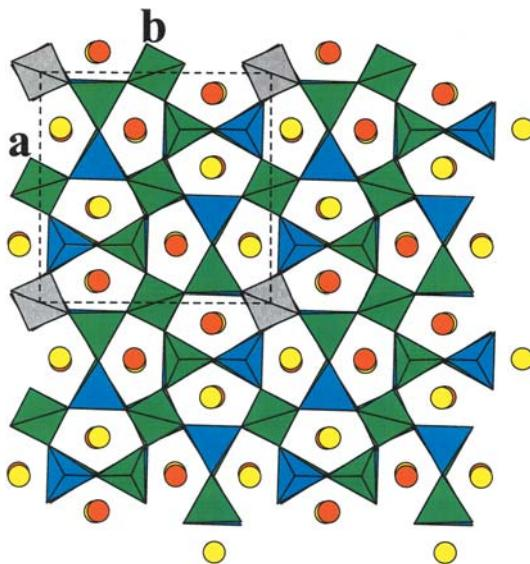
FIG. 3. The meliphanite structure projected along [001]. The  $(\text{SiO}_4)$  tetrahedra are green,  $(\text{AlO}_4)$  tetrahedra are grey and the  $(\text{BeO}_4)$  tetrahedra are blue, the Na atoms are yellow, and the Ca atoms are orange. The unit cell is outlined.  $\phi$ : unspecified anion.
