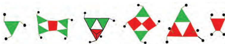
FIG. 13. The six borate clusters present as FBBs in the structures of all borate minerals. Legend as in Fig. 6.
