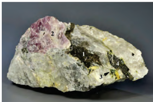
FIG. 1. General view of quartz-rich rock: pectolite aggregate (1), sogdianite (2), turkestanite (3), aegirine (4). The size of the sample is 12 cm x 9 cm x 5 cm.
