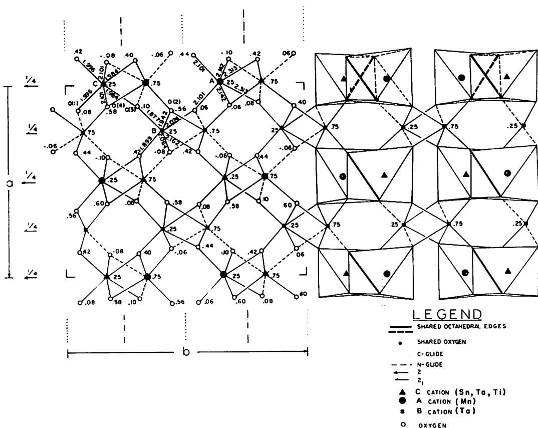
FIG. 1. Projection of the structure of wodginites along  $z$ . Prototype atoms are labelled A(=Mn), B(=Ta,Nb), C(=Sn,Ta,Ti), O(1), O(2), O(3), O(4). Shown are chains of staggered  $(A_{1/2}C_{1/2})-O$  octahedra parallel to  $z$  seen end-on; B-O octahedral chains are not shown.
