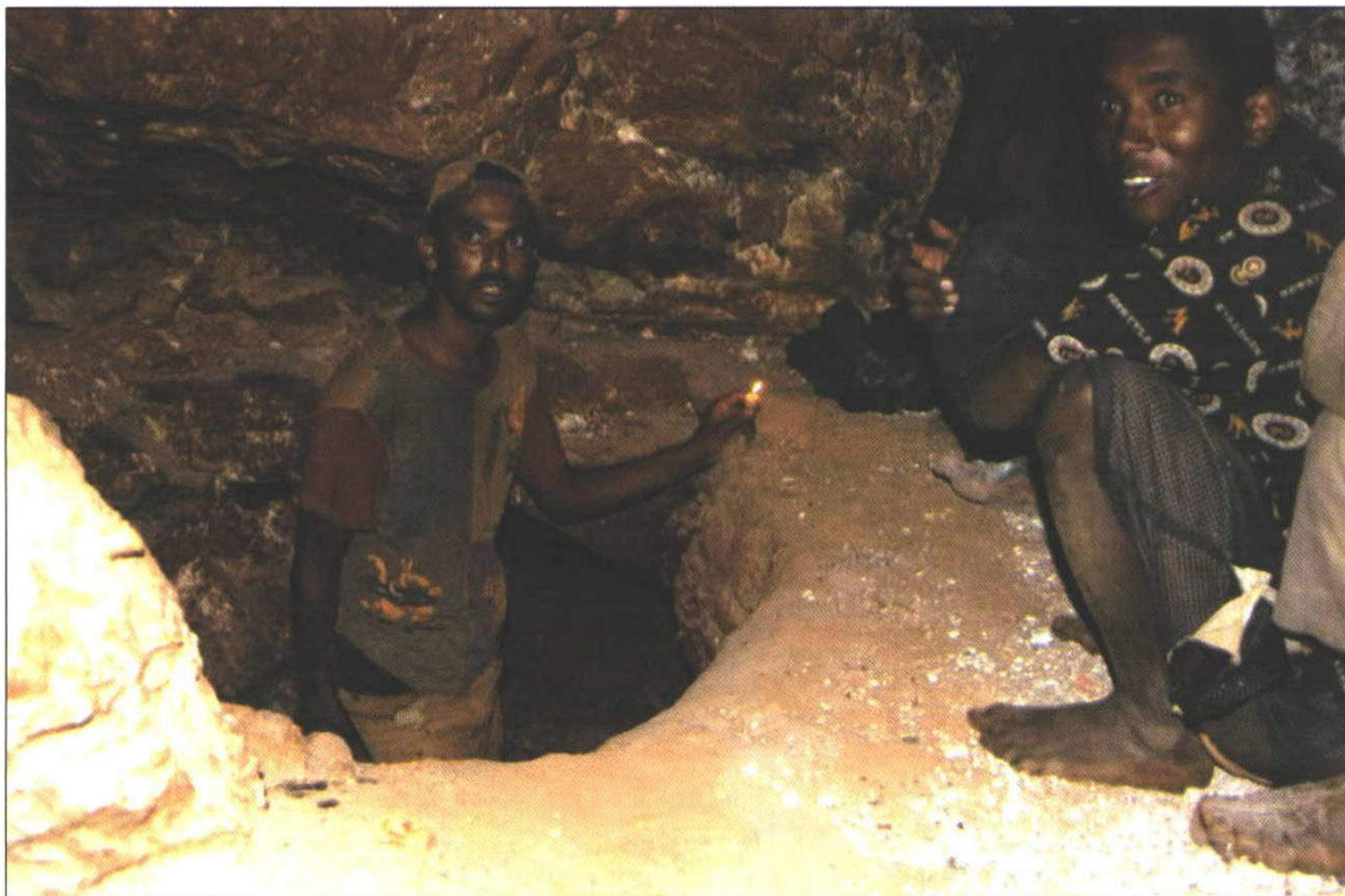
Figure 4. Mining for pezzottaite is done by candlelight using simple hand tools; this zone contained numerous vugs. Photograph by Brendan M. Laurs, GIA.
