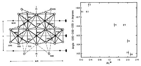
FIGS. I and 2: FIG. I (left). Diagram of oxy-kaersutite viewed along the normal to (100) showing selected portions of cell content. FIG. 2 (right). Plot of angle O(5)-O(6)-O(5) against tetrahedral aluminium content for the following Ca-rich clino-amphiboles: I. Tremolite (Papike *et al.*, 1969).
