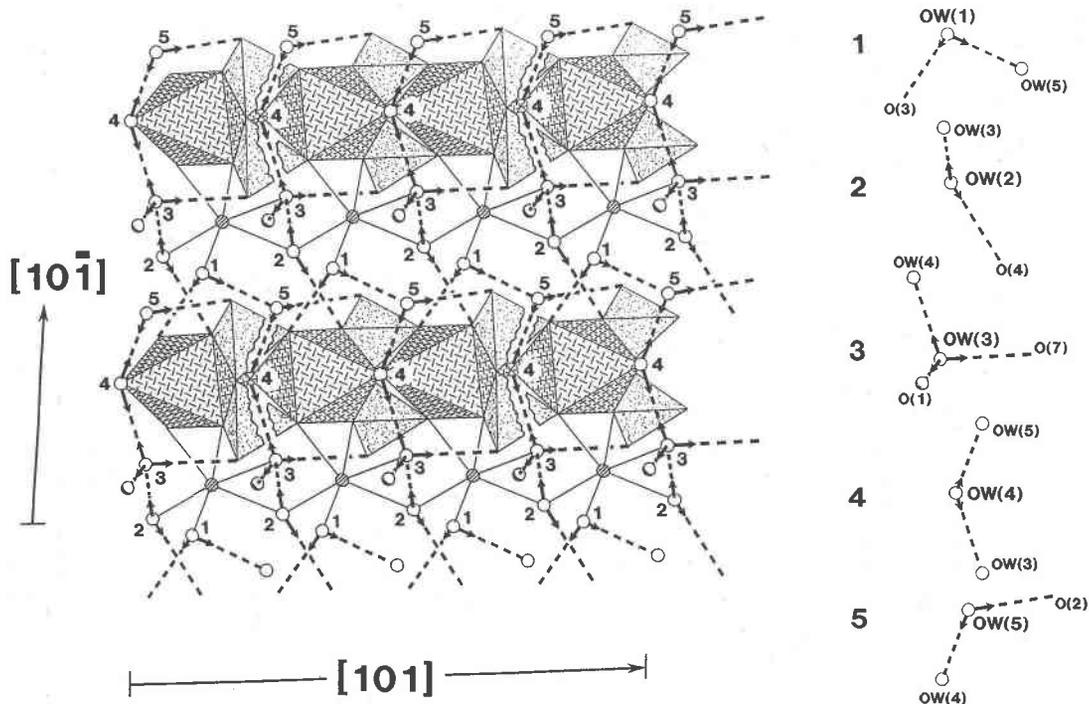
FIG. 6. The structure of woolldridgeite projected down  $[010]$  and showing the network of H-bonds; donor  $\rightarrow$  acceptor bonds are shown as heavy broken lines. Local details of each  $(\text{H}_2\text{O})$  group are shown to the right of the figure.
