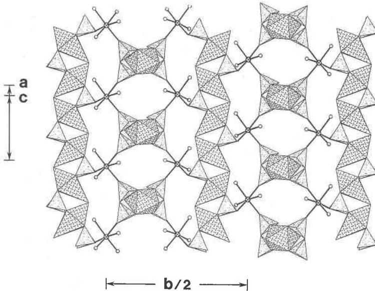
FIG. 5. The structure of wooldridgeite projected onto  $(\bar{1}01)$ , legend as in Figure 3; Na atoms (omitted for clarity) occur in the interstices between chains adjacent along  $[101]$ .
