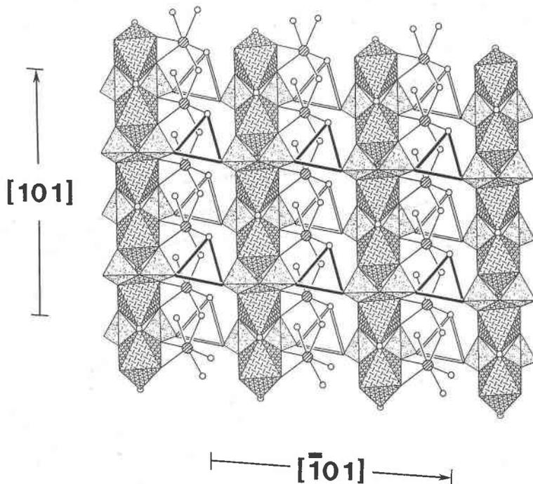
FIG. 3. Linkage of  $[\text{Cu}(\text{P}_2\text{O}_7)\phi]$  chains along  $[\bar{1}01]$  in woolldridgeite (projected down  $[010]$ ); polyhedral shading as in Figure 1, small unshaded circles are  $(\text{H}_2\text{O})$  groups, and  $\text{Na}-\text{O}$  bonds are shown as thin lines, the heavily drawn triangles are faces of  $(\text{Ca}\phi_6)$  octahedra above the plane of the sheet, and the double-line triangles are faces of  $(\text{Ca}\phi_6)$  octahedra below the plane of the sheet.
