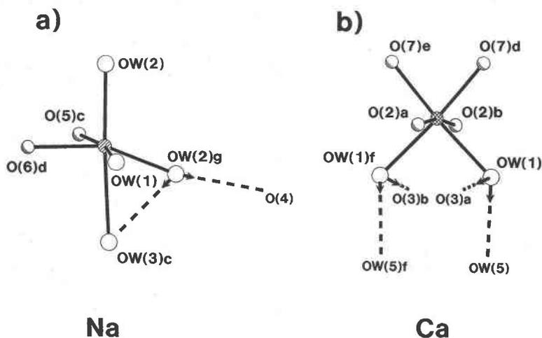
FIG. 1. The coordination of the interstitial-cation sites: (a) Na (diagonal-shaded circles); (b) Ca (cross-hatched circles); highlighted circles are O atoms, larger unshaded circles are (H<sub>2</sub>O) groups, donor  $\rightarrow$  H bonds are shown as arrows, H  $\rightarrow$  acceptor bonds are shown as broken lines.
