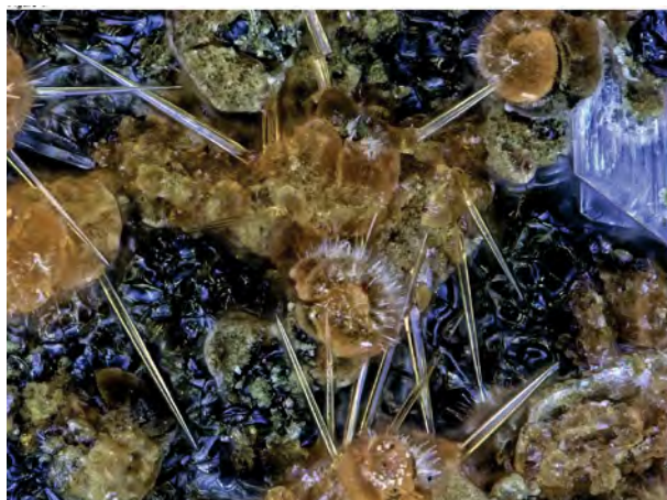
FIGURE 1. Caseyite needles with gypsum and orange-yellow balls of another potentially new Al-V-S-O-bearing mineral; holotype specimen (no. 73526) from the Packrat mine; FOV 0.68 mm across. (Color online.)
